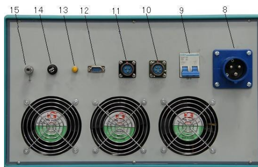
Figure 4-1b back panel of control box
